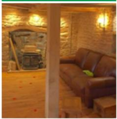
John and Hannah were busy during lockdown. Hannah has stripped the walls and repointed the stonework using lime mortar. John has made supporting beams from an oak tree that was felled on the park, and has replaced the floor with one made from an old squash court. They have also replaced the ceiling, and the floor in the bedroom above.
